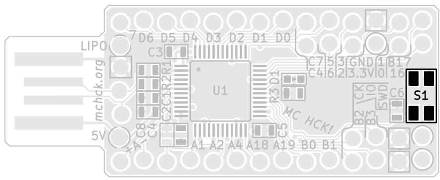
This **pushbutton switch** lets you change the microcontroller into a "bootloader" mode where it will accept a new program.
