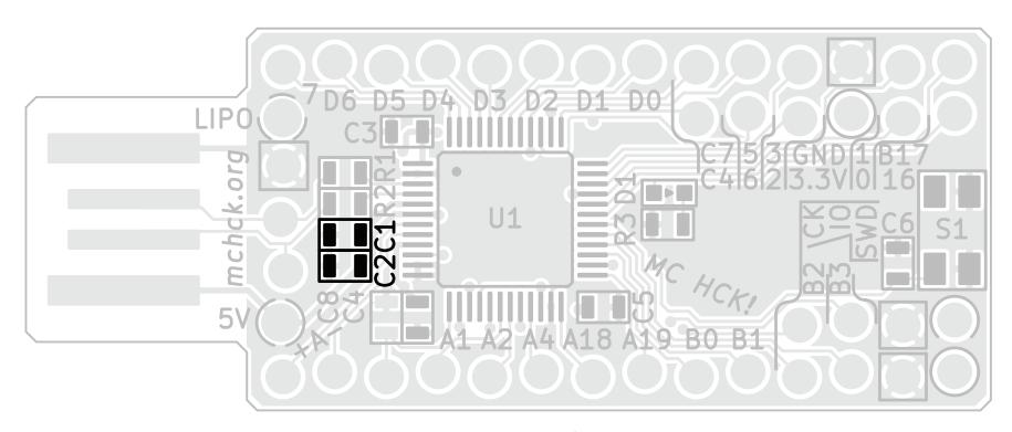
**Bulk capacitors** act as larger reservoirs of current close to power hungry components, preventing brown-out when
