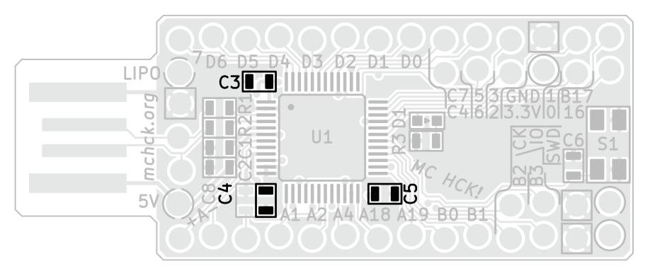
**Bypass** or **decoupling capacitors** reduce digital switching noise by providing a small reservoir of fast-reacting current close to a potentially noisy digital chip to smooth out sudden changes in current draw.
