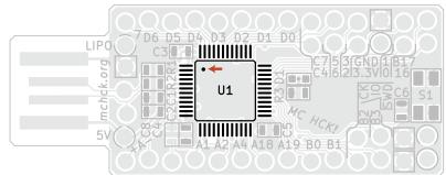
The microcontroller is the brain of the operation. It has a ton of different features all on a single tiny silicon chip. This chip, a Freescale Kinetis MK20DX128, is an ARM microcontroller, similar to but less powerful than the CPU in your phone or tablet. Note the *alignment dot*.
