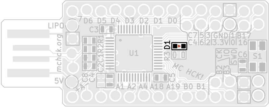
This **light emitting diode** is like a tiny light bulb that glows when you pass curent through it. Note the **direction arrow** (on the back in green) if you put it in backwards, it won't light up!
