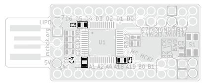
Bypass or decoupling capacitors reduce digital switching noise by providing a small reservoir of fast-reacting current close to a potentially noisy digital chip to smooth out sudden changes in current draw.
