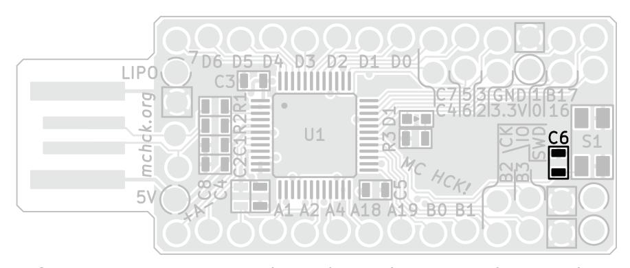
**Debouncing** capacitors smooth out chatter that occurs when a push-button switch is pressed, preventing false triggering.
