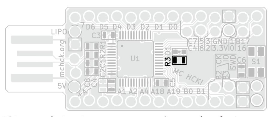
This **current limit resistor** prevents too much current from flowing through the LED, which could cause it to fail.
