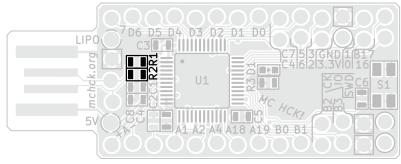
**Termination resistors** prevent electrical reflections in the USB cable that might cause the host computer to incorrectly call a 1 versus a 0. The black side is normally placed facing up.
