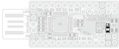
Debouncing capacitors smooth out chatter that occurs when a pushbutton switch is pressed, preventing false triggering.
