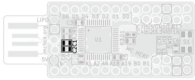
**Bulk capacitors** act as larger reservoirs of current close to power hungry components, preventing brown-out when
