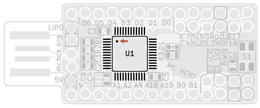
The **microcontroller** is the brain of the operation. It has a ton of different features all on a single tiny silicon chip. This chip, a Freescale Kinetis MK20DX128, is an ARM microcontroller, similar to but less powerful than the CPU in your phone or tablet. Note the *alignment dot*.
