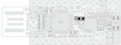
This **light emitting diode** is like a tiny light bulb that glows when you pass curent through it. Note the *direction arrow* (on the back in green) if you put it in backwards, it won't light up!
