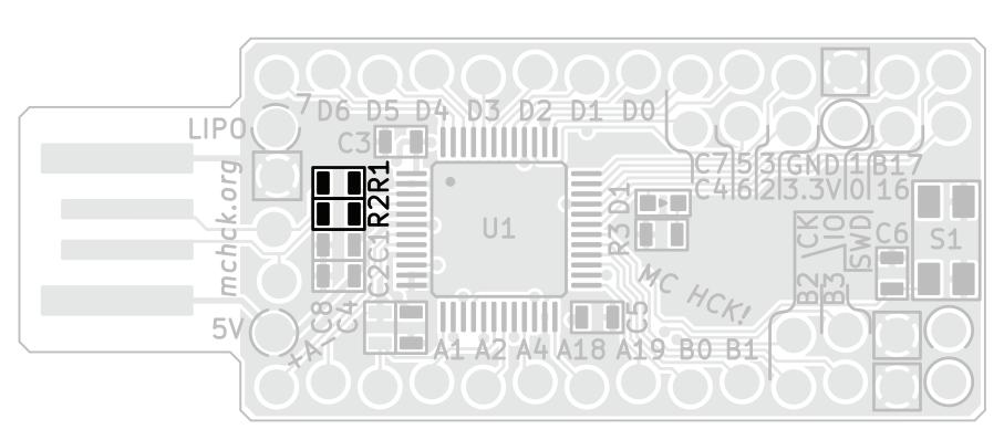
**Termination resistors** prevent electrical reflections in the USB cable that might cause the host computer to incorrectly call a 1 versus a 0. The black side is normally placed facing up.
